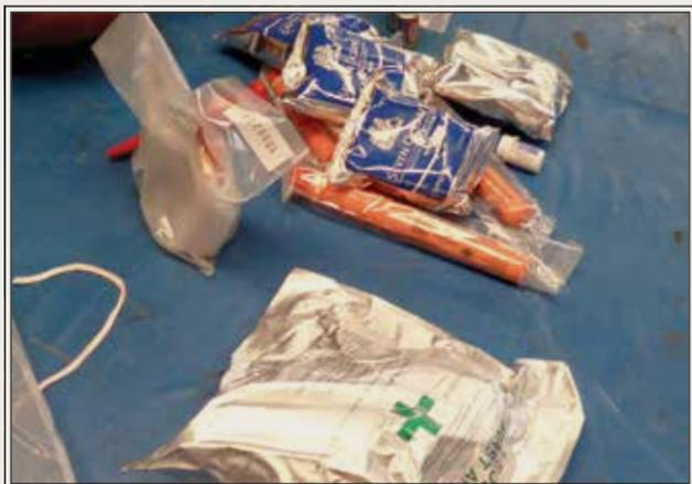
**When your raft is out of its canister or valise during servicing, you can check out all of its neatly packed components (top). In the water, ballast bags will fill and help stabilize the raft (center). During the inspection, expired flares, medicine and food rations are replaced (bottom).**
