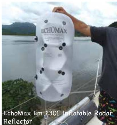
EchoMax Em 2301 Inflatable Radar Reflector
